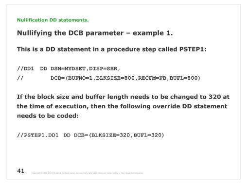
The values of the DSN and DISP parameters and the BUFNO and RECFM subparameters remain unchanged.
