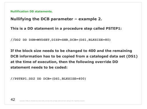
If the DCB parameter is being modified and a DCB positional subparameter needs to be retained, the positional subparameter must be coded. This applies whether the positional subparameter exists on the DD statement in the procedure definition or not.
