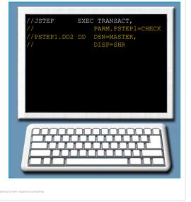
The code on the right represents the EXEC statement used to invoke the procedure.
