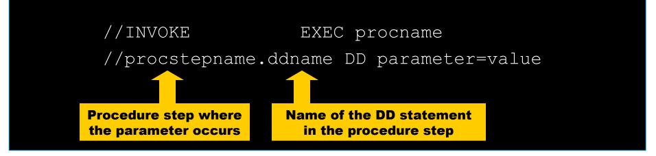
The DD statement has a two-part name. It consists of the name of the procedure step in which the DD statement to be changed occurs, followed by a period and the name of the DD statement in the procedure step.
