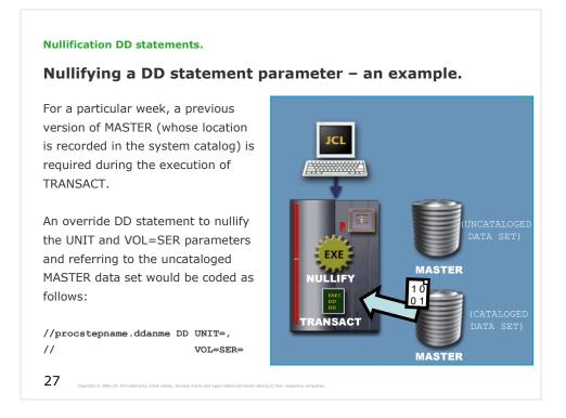
The code will nullify the UNIT and VOL=SER parameters specified for the data set in the procedure definition and the system will go to the cataloged data set by default.
