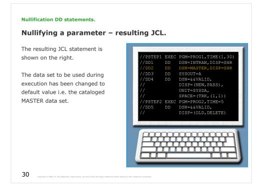
The parameter DISP=SHR, specified for DD2 in the procedure definition, is retained because the existing DD statement keyword parameters, that are not overridden, are retained.
